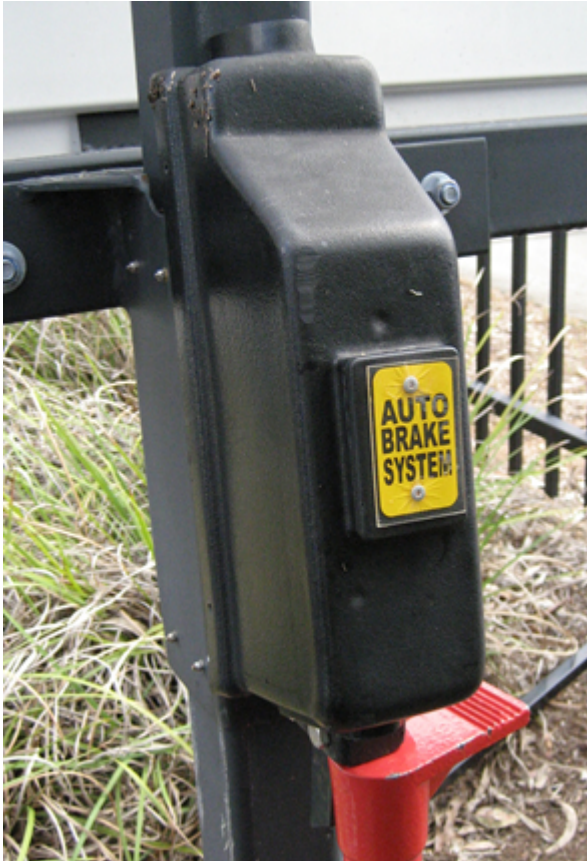
Photograph 6 - Emergency brake cover on one kind of winch type sign. It is important to inspect the inside mechanism as critical faults could be concealed by the cover.
