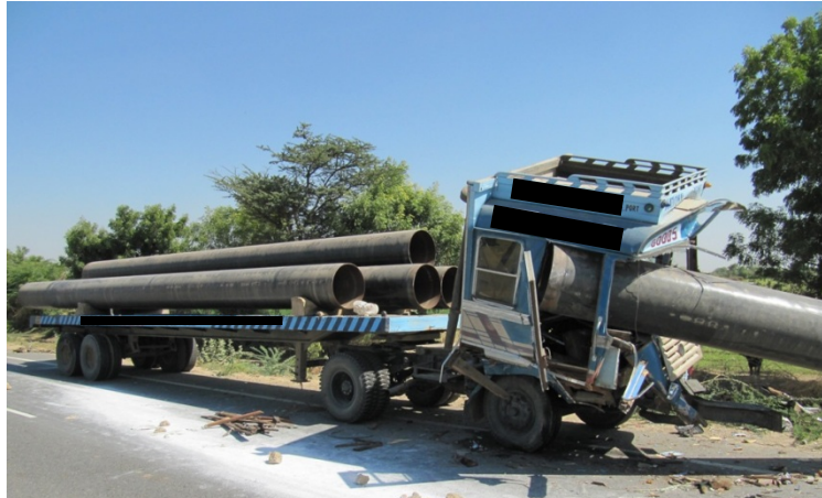
Truck after breaking hard and unsecured pipe travelled forward
